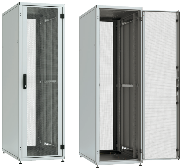
Server cabinet 42U, width 600 mm x depth 1000 mm Front- and rear door steel, perforated, 1-part with turning handle
