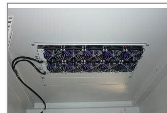
„Silent“-Fans installed in Inner Roof
