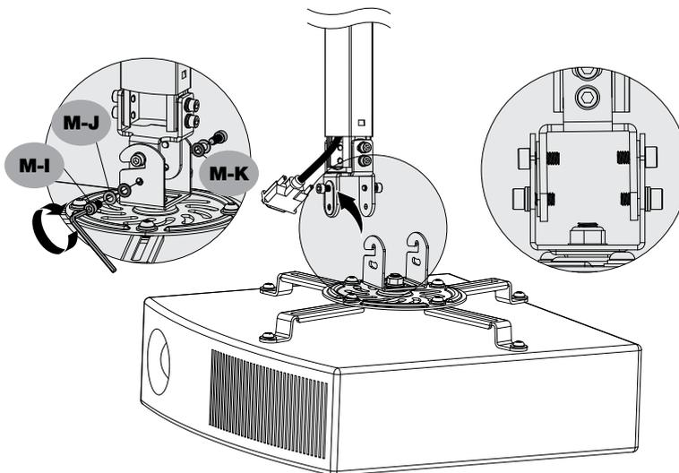
**EN Hanging the Projector onto the Assembled Pivot Bracket**
