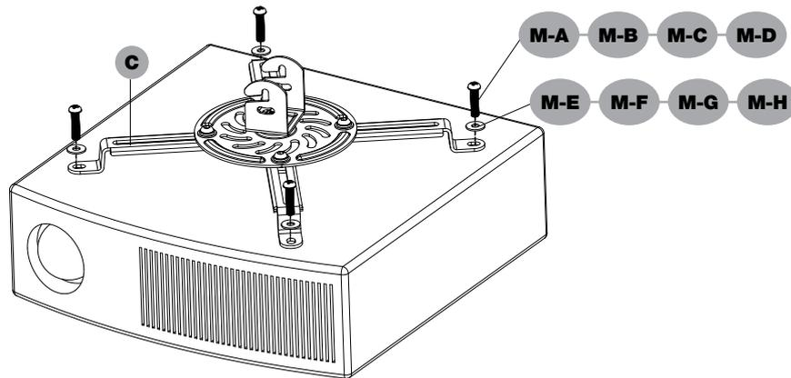
**EN Installing the Adapter Bracket**
